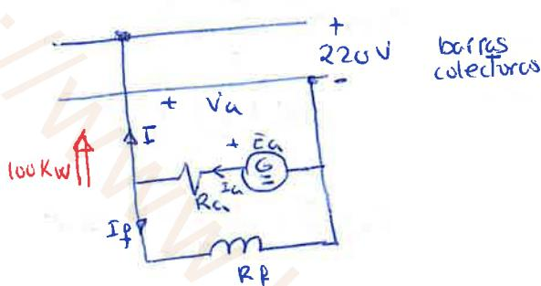
$$\bullet E_a = \frac{P}{\alpha} 2N\phi = \frac{P}{2\pi f} 2\pi\phi$$
