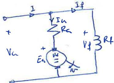
$$\text{en régimen de vacío: } I_f = \frac{V_u}{R_f} = \frac{250}{250} = 1 \text{ A}$$
