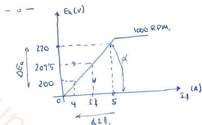
$$I_f = \frac{V_f}{R_f} = \frac{V_u}{R_f} = \frac{220}{40} = 5'5A.$$
