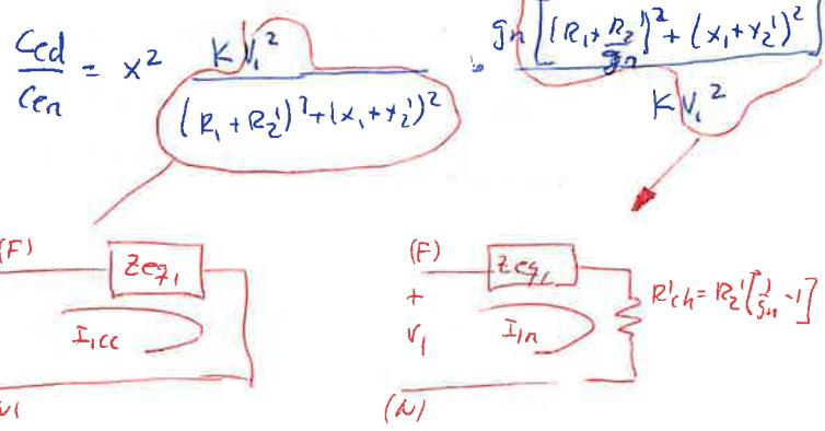
$$\frac{C_{ed}}{C_{en}} = x^2 \left[ \frac{I_{cc}}{I_{in}} \right]^2 g_n = \left( \frac{1}{\sqrt{2}} \right)^2 4^2 \cdot 0.025 = \underline{0'2}$$
