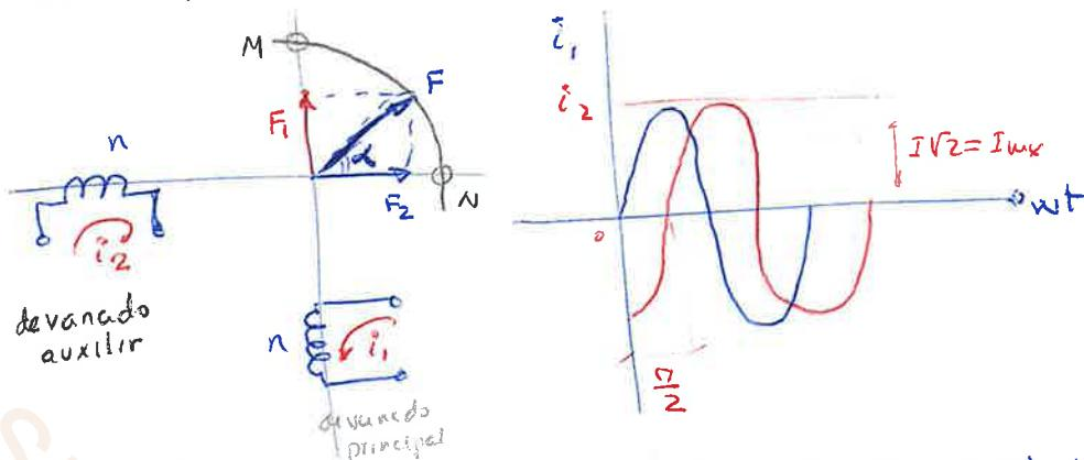
$$\begin{aligned} i_1 &= I_{max} \sin \omega t \rightarrow F_1 = n i_1 = n I \sqrt{2} \sin \omega t = F_{max} \sin \omega t \\ i_2 &= I_{max} \cos \omega t \rightarrow F_2 = n i_2 = n I \sqrt{2} \cos \omega t = F_{max} \cos \omega t \end{aligned} \quad \left. \right\} \Rightarrow$$
