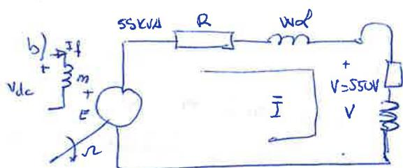
$$\bar{E} = \bar{V} + \bar{Z} \cdot \bar{I} \quad I = \frac{S}{V} = \frac{55 \cdot 10^3}{550V} = 100A.$$
