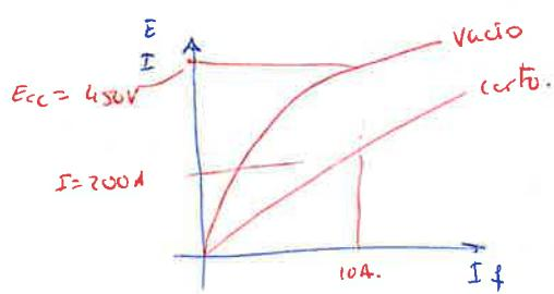
$$\text{a)} \quad \bar{Z} = \frac{E_{cc}}{I} = \frac{450}{200} = 2'25\Omega \quad \text{impedancia sincrónica.}$$
