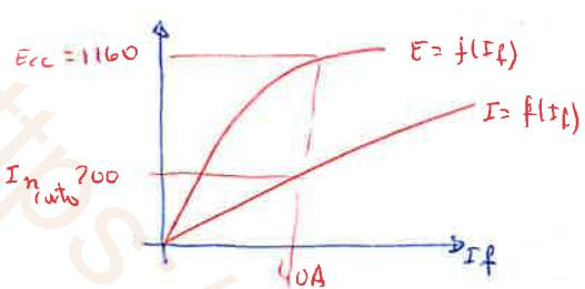
$$\bar{Z} = \frac{E}{I_{\text{cortocircuito}}} = \frac{1160}{200} = 5'80\Omega \quad \text{impedancia sincrónica.}$$
